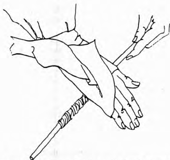
A scrap of leather, made into a cuff, does the same job in puni-making as the paddle
